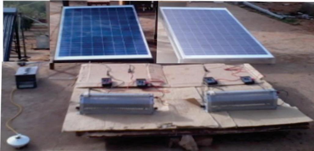
Figure 1: Relief Photo of the Experimental Set-up of the cleaned and dusty PV modules
