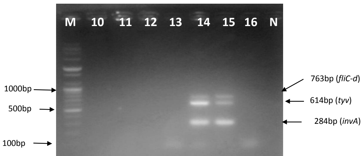
Plate II: Electrophoresis Gel Picture of mPCR Amplified invA , tyv and fliC-d Genes of Isolates from GK and YD.
