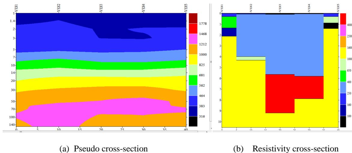
Figure 6: (a) Pseudo cross-section and (b) Resistivity cross-section of VES 1-5 along profile 5 in Masallachi Idi Dumpsite.
