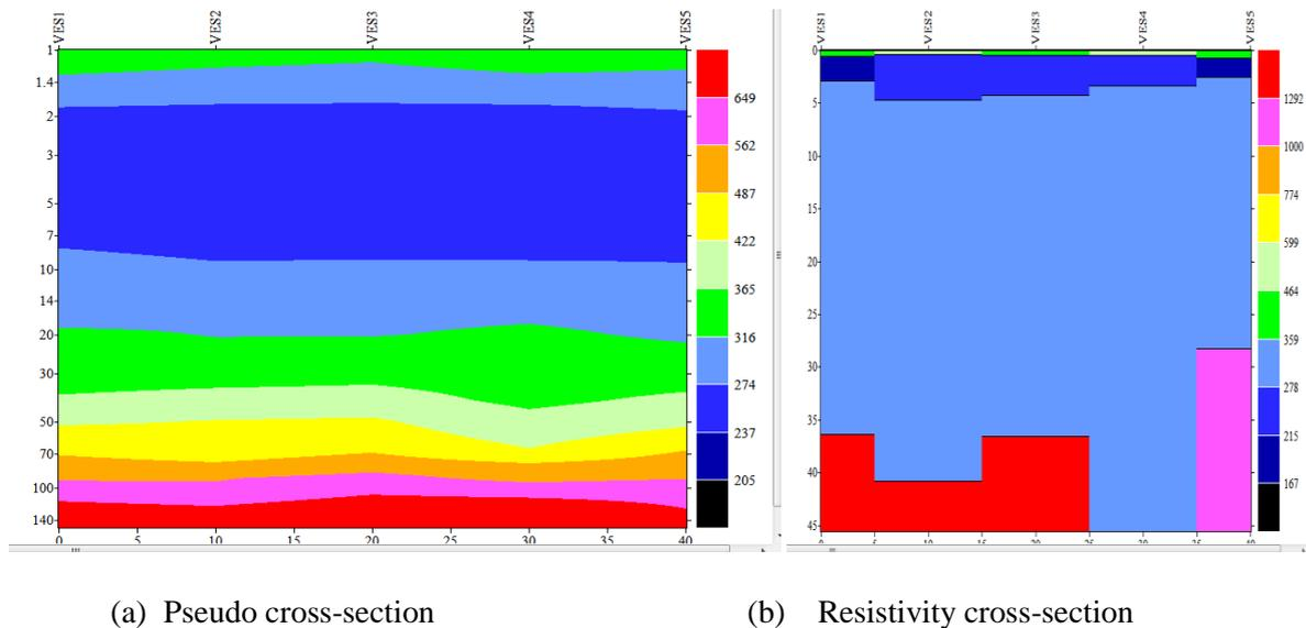
Figure 5: (a) Pseudo cross-section and (b) Resistivity cross-section of VES 1-5 along profile 4 in Masallachi Idi Dumpsite
